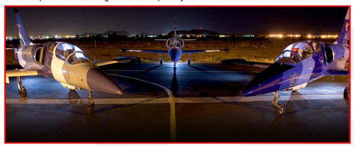
The tall, swept vertical tail has an inset rudder. Variable-incidence horizontal stabilizers with inset elevators are mounted at the base of the rudder and over the exhaust nozzle. Side-by-side airbrakes are located under the fuselage ahead of the wing's leading edge. Flaps, landing gear, wheel brakes and air brakes are powered by a hydraulic system. Controls are pushrod-actuated and have electrically powered servo tabs on the ailerons and rudder.
